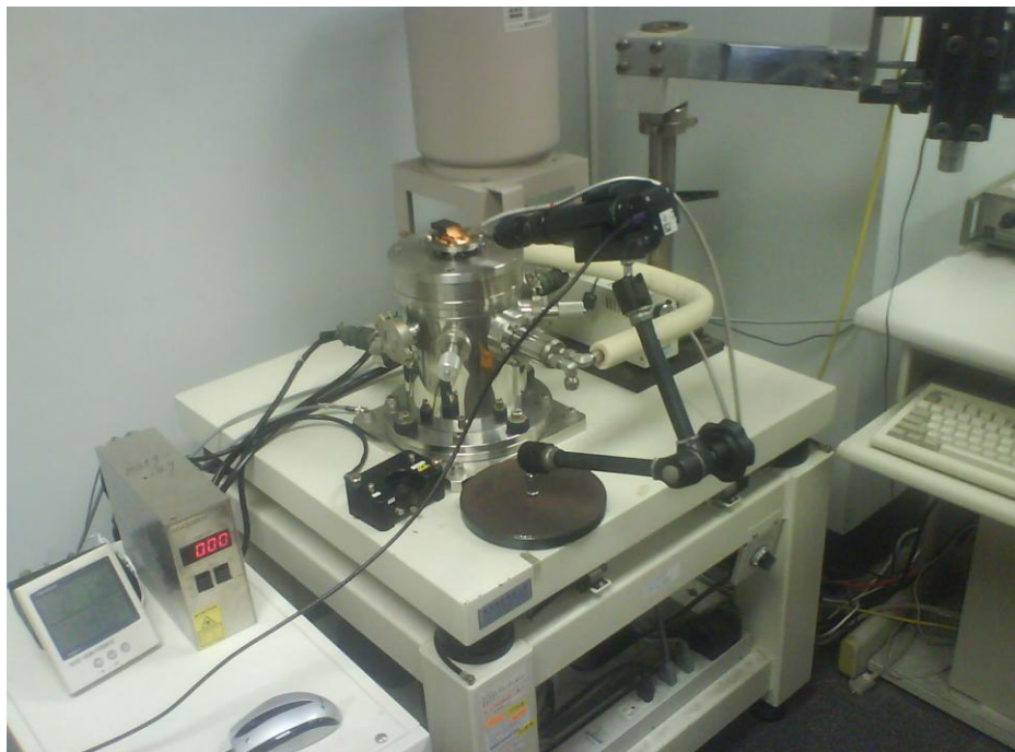
Figure 7. The combined system of an AFM and a nanotester for forces measurements in two directions.
