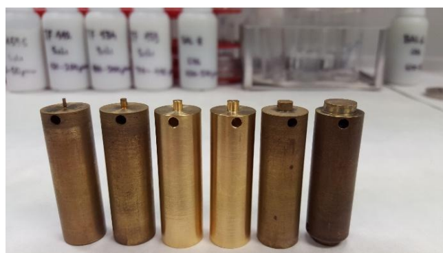
Fig. 5b – inserts with different lenght of heating zone
