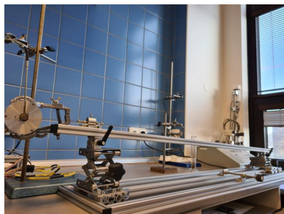
Fig. 5d – guide track finely adjustable in all axes
