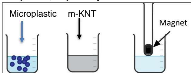
**Figure.3.5** Schematic representation of m-CNT addition and magnetic removal from aqueous suspension containing microplastics.
