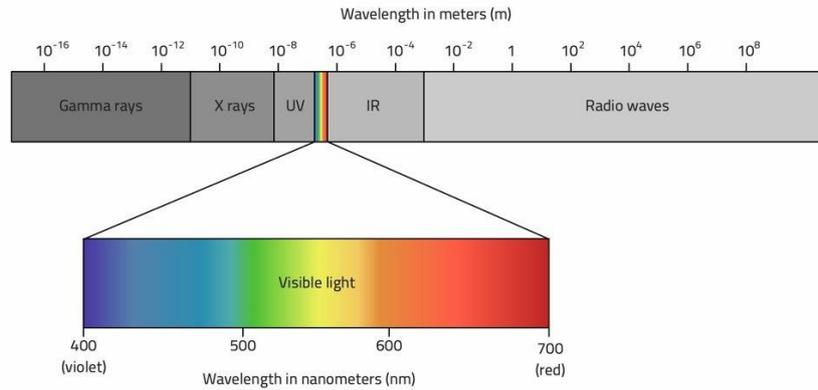
**Figure 2.2** Electromagnetic spectrum (Aksoy, 2016).
