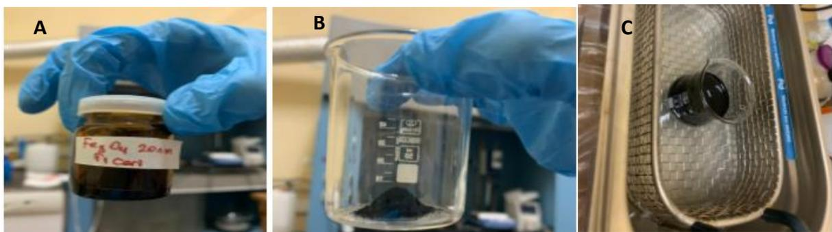
**Figure.3.3** a) Fe<sub>3</sub>O<sub>4</sub> NP, b) 200 mg CNT-COOH c) CNT-COOH ve Fe<sub>3</sub>O<sub>4</sub> NP in Ultrasonic bath
