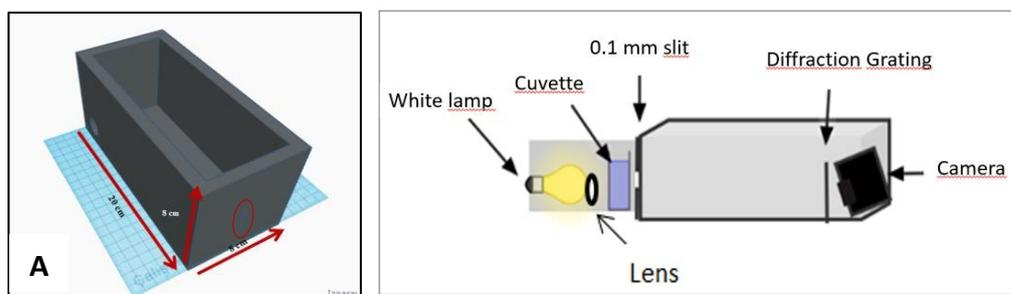
**Figure.3.1** a) The 3D design of the spectrometer that has been made with TinkerCad, b) Schematic representation of the spectrometer(Original).
