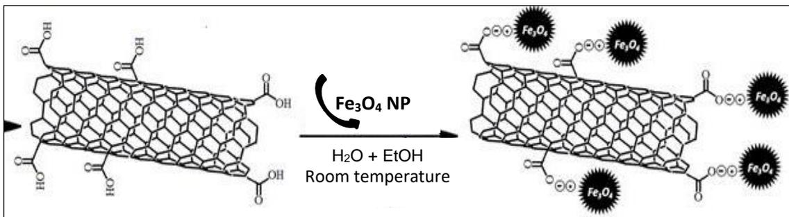
**Figure.3.2** m-CNT 's synthesis reaction (Sadegh vd., 2014; Sadegh vd., 2018).
