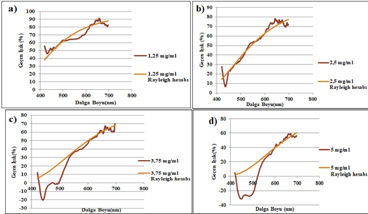
**Figure.4.5** Transmission of light through different concentrations of coffee solutions and Rayleigh scattering calculations. a) 1,25 mg/mL b) 2,5 mg/mL c) 3,75 mg/mL d) 5 mg/mL
