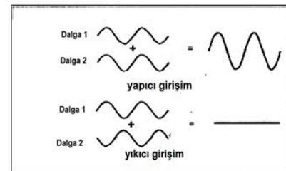
**Figure.2.3** Constructive and destructive interference (Korkmaz, 2013)
