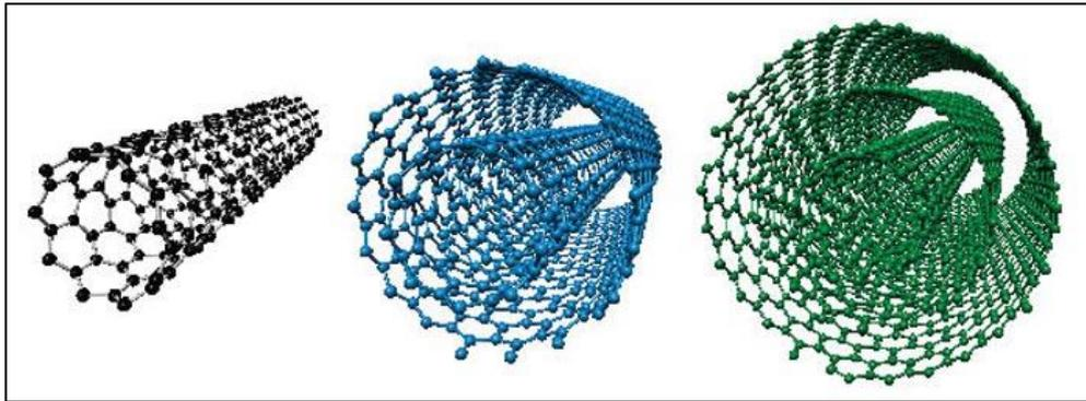
**Figure.2.9** Carbon nanotubes single, double and three-walled. (Dumé, 2013).
