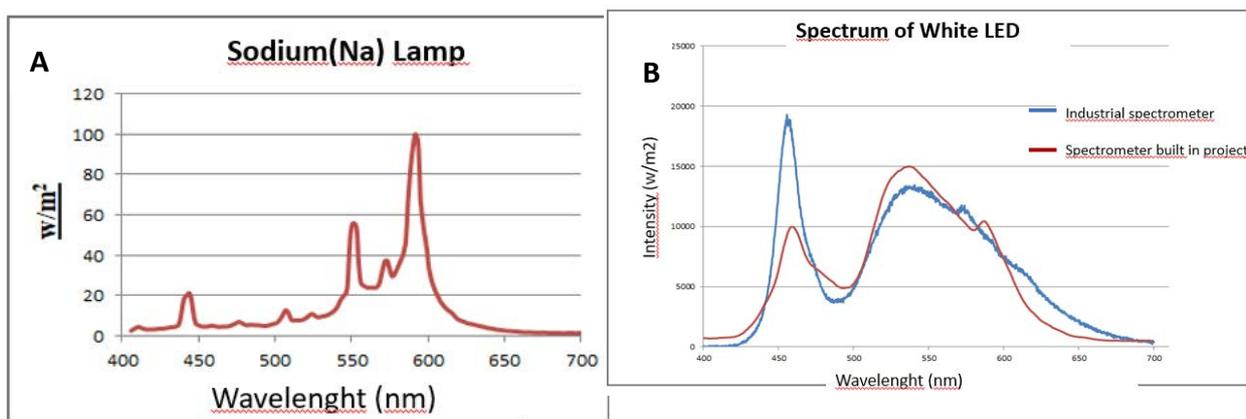
**Figure.4.2** Spectrum of the sodium lamp, b)Comparison of the White LED s spectrum taken with an industrial spectrometer.
