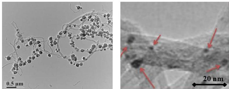
**Figure 2.10.** Image of synthesized material of CNT and  $\text{Fe}_3\text{O}_4$  NP's at electron microscope (TEM) (Saber-Samandari vd., 2016; Sadegh vd., 2018).
