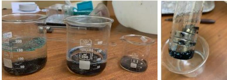
**Figure.4.6** A)Steps of Magnetic Separation. B) The picture of accumulated microplastics on the magnet after the magnetic separation from the water.
