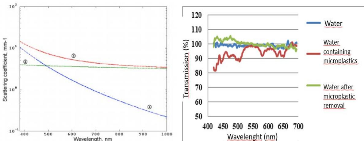
**Figure.4.8** A)Rayleigh scattering (1),Mie scattering (2),Combination of Mie and Rayleigh scattering equations (3) (Petrov,2012). B) Transmission display chart where before and after plastics were removed from water.
