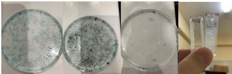
**Figure.4.7** A) The sample containing HDPE microplastics B) Suspension where m-CNT is added. C) Sample after the microplastics are removed D) Cuvettes with samples before and after the microplastic removal.
