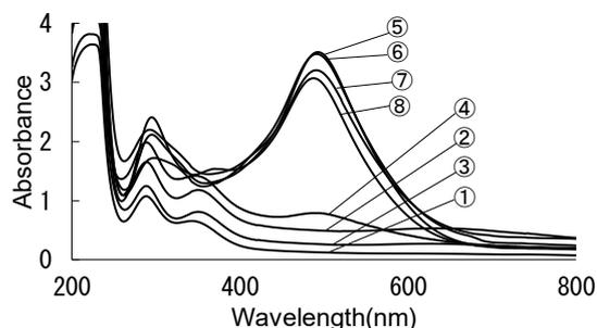
Fig.3 ABS spectra of iodine color reaction of PVA with boric acid
