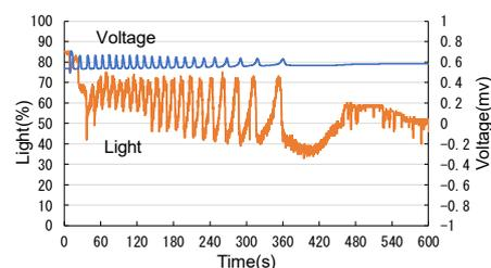
Fig.6 Observed oscillation of the BR reaction that PVA ⑧ was added instead of starch
