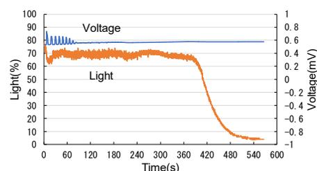
Fig.5 Observed oscillation of the BR reaction that PVA ① was added instead of starch
