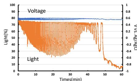
Fig.8 Observed oscillation of the BR reaction with starch in the presence of ferricyanide
