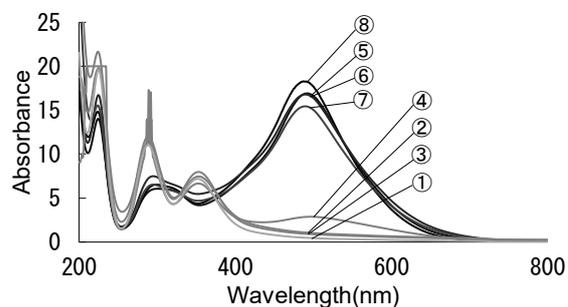
Fig.2 ABS spectra of PVA-iodine color reaction solutions
