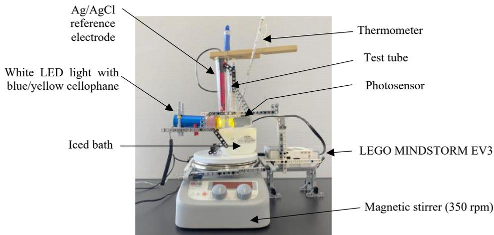
Fig. 1 Equipment for measurement of BR reaction
