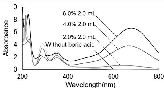
Fig.4 Iodine color reaction of PVA ① with various concentrations of boric acid
