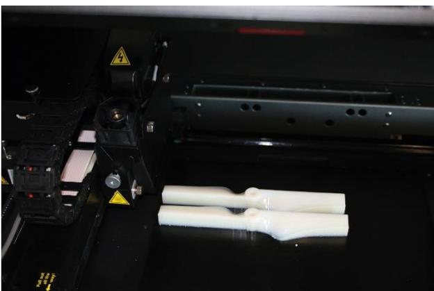
Figure 12: *Design I* after completion of the 3D printing process
