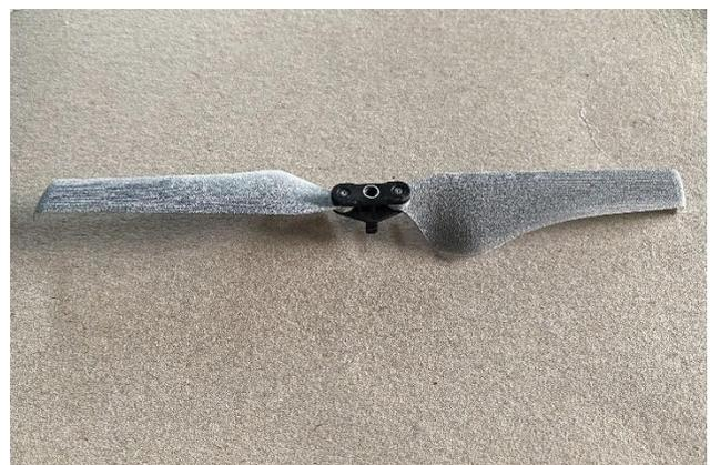
Figure 15: *Design II* with sloped winglets
