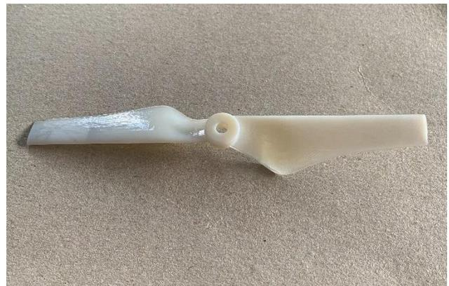
Figure 14: *Design I* with connection piece for test rig
