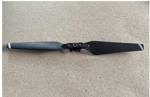
Figure 13: Standard rotors of the Mavic Pro (DJI)
