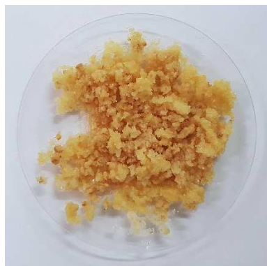
photo 4 hydrolysed Plexiglas
