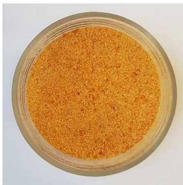
photo 5 hydrolysed Plexiglas and treated with HCl
