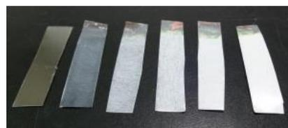
Fig.4. In air at 800°C (Ta plate) for 2, 5, 7, 9 and 12 min.
