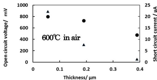
Fig.13. Property of Ta<sub>2</sub>O<sub>5</sub> thin film borned in air at 600°C, Xe lamp irradiation
