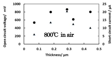
Fig.14. Property of Ta<sub>2</sub>O<sub>5</sub> thin film borned in air at 800°C, Xe lamp irradiation
