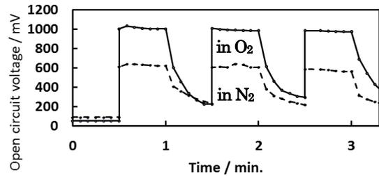
Fig.12. Light response of Ta<sub>2</sub>O<sub>5</sub>/Ta. irradiation of Xe lamp
