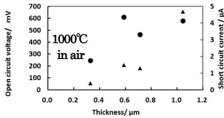
**Fig.15.** Property of  $\text{Ta}_2\text{O}_5$  thin film burned in air at  $1000^\circ\text{C}$ , Xe lamp irradiation
