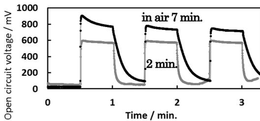
Fig.11. Light response of Ta<sub>2</sub>O<sub>5</sub>/Ta. in air and irradiation of Xe lamp
