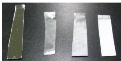
Fig.3. In air at 600°C (Ta plate) for 10, 20 and 30 min.
