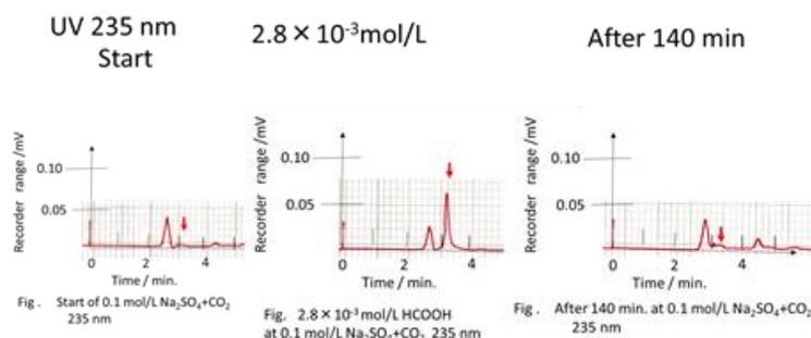
Fig.26. HPLC detected at 235 nm
